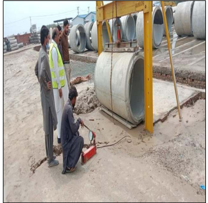
Picture 18: Lot-4 Three-Edge Bearing Test being Supervised
