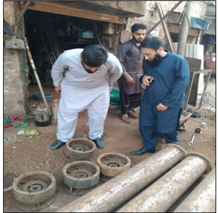
Picture 10: Inspection of Mechanical Components of Tube well for Replacement/Rehabilitation
